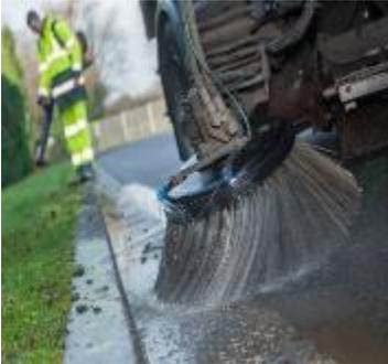
**Project will provide for an intensive removal of compacted sediments that reside within the curb areas of all citywide streets. The compacted sediments will be removed so as not to further impact deposition of the storm sewer system and adjacent drainage ways.**
